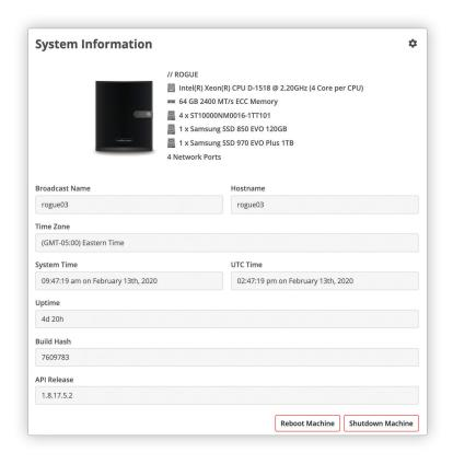
Part of the reason for this is the massive amount of RAM in the //ROGUE (more on that later). With that many streams you may get a "bump" as the media starts pulling from the RAID, but it efficiently transfers the streams to a RAM buffer so that ultimately it's streaming from RAM rather than directly from the spinning disks. I found that with the footage in the RAM buffer I could rapidly scrub several seconds of those 6 streams back and forth without a glitch.
